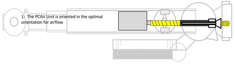
2: If the bridge does not have an under-cab GPU, the system can be mounted under the cab.
