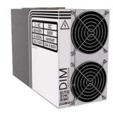
The inverter is built in 3-level structure with silicon carbide semiconductor. This allows a very high switching frequency, whereby very compact passive components (chokes, capacitors) can be selected. Due to the high-power density a module has only 11 lb ( $\approx$  5 kg). Therefore, the entire active part at 90 kVA output power with 8 modules has only 88 lb ( $\approx$  40 kg).
